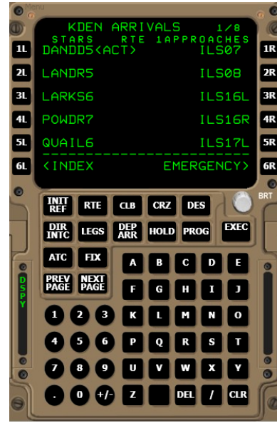
Figure 8: The display for the Flight Management Computer showing the Departures/Arrivals page for Denver (KDEN). The emergency prompt appears next to button 6R at the lower right.
