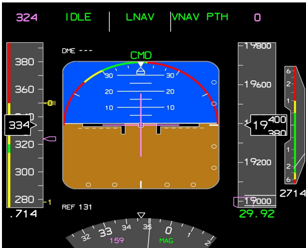
Figure 7: The Primary Flight Display (PFD) showing bank angle, pitch, airspeed, vertical speed, altitude and heading.
