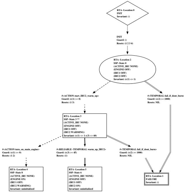
Figure 3: The timed automaton model corresponding to Figure 2.
