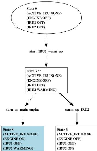
Figure 2: The beginning of a state space plan for Saturn Orbit Insertion.
