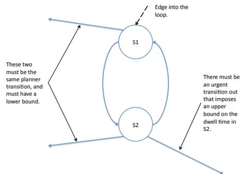
Figure 6: An illustration of the subgraph pattern that provides candidates for loop acceleration in CIRCA.
